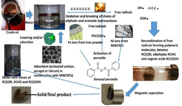
Figure 1. Scheme for oxidation and solidification of crudr petroleum.
